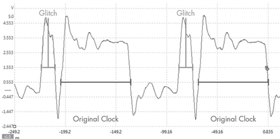
Clock XORd with Glitch Width = 10% Offset = -15%
