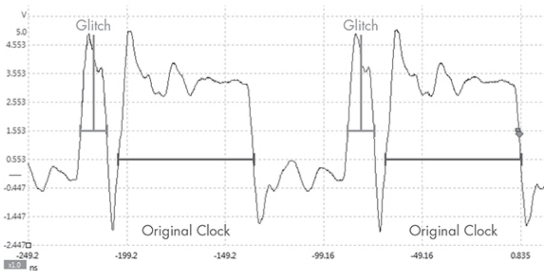
Clock XORd with Glitch Width = 10% Offset = -15%
