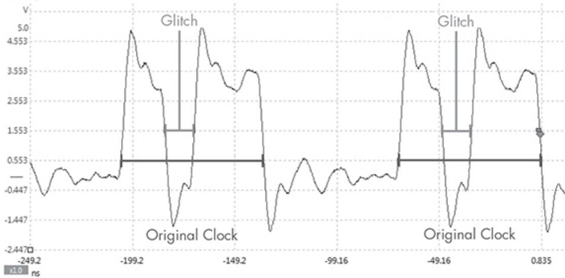
Clock XORd with Glitch Width = 10% Offset = +15%
